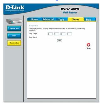
The Diagnostics window allows users to test the functionality of the router by executing a ping test. Enter the IP address of the Ping Target and then click **Test**.
